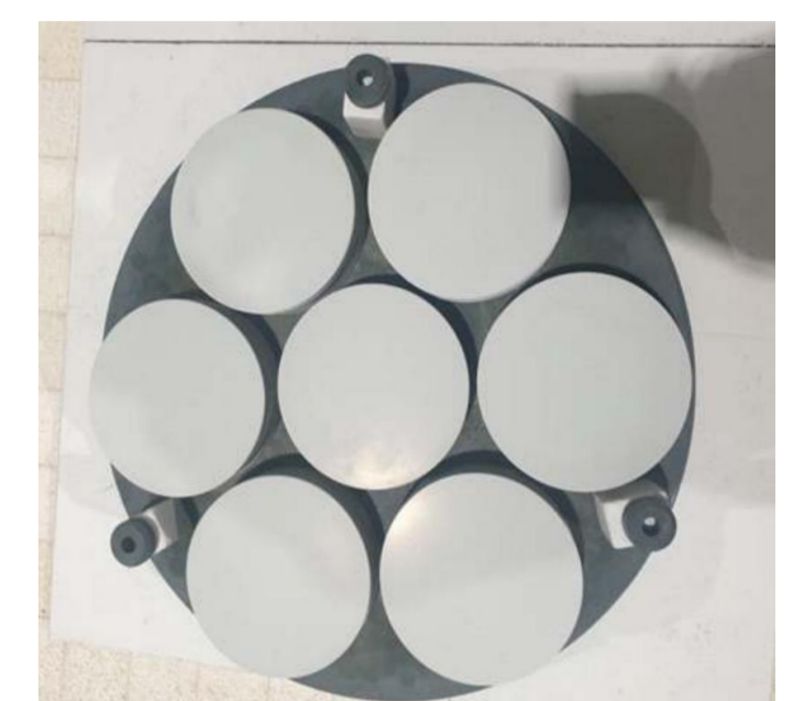
Fig. 10. Prototype of a debound body produced using the optimized debinding process for \text{Si}_3\text{N}_4 .
