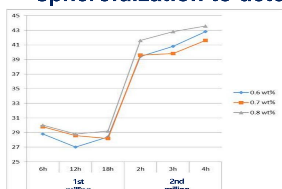
Fig. 5. Viscosity as a function of dispersant content and milling time (unit: cP).
